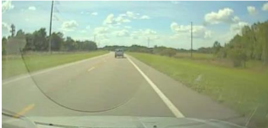
Subject vehicle not considered to be following forward vehicle (Image source: UMTRI RDCW dataset)
